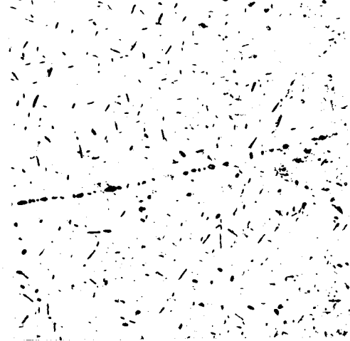
Figure 43. 33.9% vanadium (Series I) arc melted and annealed 30 hours at 910° C, 96 hours at 500° C and water quenched. Beta matrix with second phase apparently alpha. Unetched. X 250
