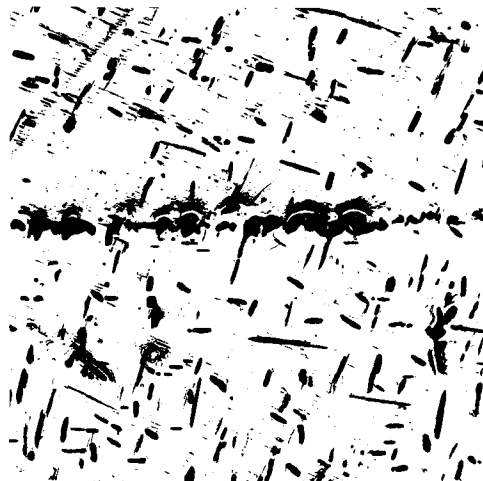
Figure 31. 20% vanadium (Series II) arc melted and homogenized at 1200° C 16 hours, heated at 900° C for 14 hours, 80 hours at 700° C and water quenched. Primary alpha in partly retained beta. Some impurity phase. Etchant 1 HNO 3 (conc), 1 HF (48%) 3 glycerol. X 250
