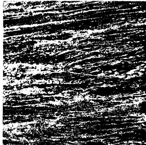
Figure 67. 69.5% vanadium hot rolled at 800° C to 66% reduction. Alloy strip bent. Etchant 2 HNO 3 (conc), 1 HF (48%), 3 glycerol. X 250
