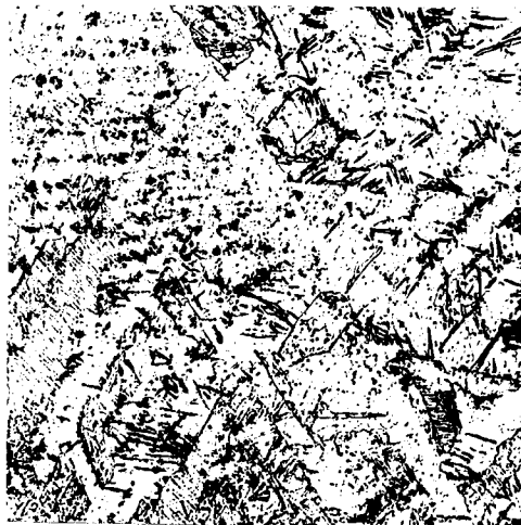
Figure 11. 1.2% vanadium (Series II) as-arc-melted alloy. Etchant 1 \text{HNO}_3 (conc), 1 HF (48%), 3 glycerol. X 250
