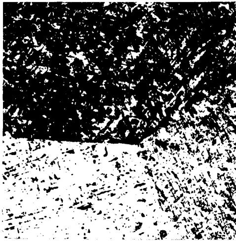
Figure 13. 7.6% vanadium (Series II) as-arc-melted showing partial transformation of beta phase on quenching. Etchant 1 HNO 3 (conc), 1 HF (48%), 3 glycerol (by volume). X 250
