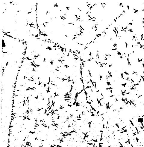
Figure 15. 69.5% vanadium (Series II) as-arc-melted showing retained beta phase second phase of impurity or slight inhomogeneity. Etchant 2 HNO 3 (conc), 1 HF (48%), 3 glycerol. X 250
