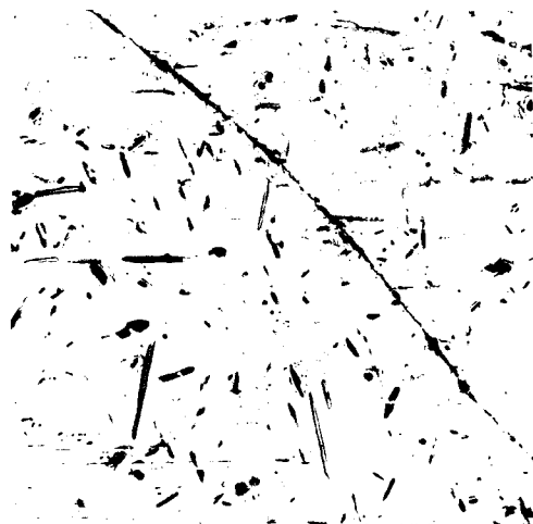
Figure 40. 14.1% vanadium (Series I) arc melted and annealed at 910° C for 36 hours at 750° C before water quenching. Primary alpha in partly retained beta background. Etchant 1 HNO 3 (conc), 1 HF (48%), 3 glycerol. X 250
